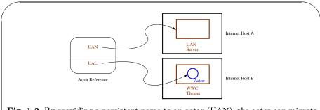
Fig. 1.2. By providing a persistent name to an actor (UAN), the actor can migrate from a host to another without breaking existing references.
