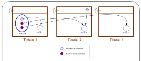
Fig. 1.5a. Before migration of actor m from Theater 1 to Theater 2, its references to actors b and c are remote, while its reference to actor a is local.
