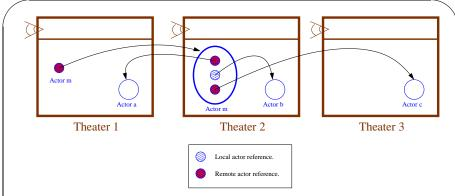
Fig. 1.5b. After migration of actor m, its reference to actor a becomes *remote* and its reference to actor b becomes *local*. Its reference to actor c remains unchanged. A temporary forwarder for actor m is left in Theater 1.
