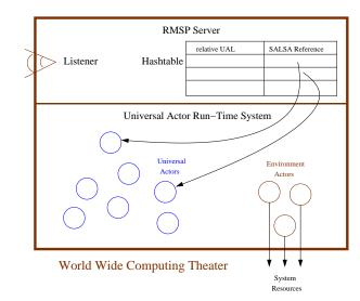
**Fig. 1.4.** A WWC Theater provides runtime support to Universal Actors. A Theater contains: (1) a RMSP server with a hashtable mapping relative UALs to actual Salsa actor references, and (2) a runtime system for universal and environment actors.
