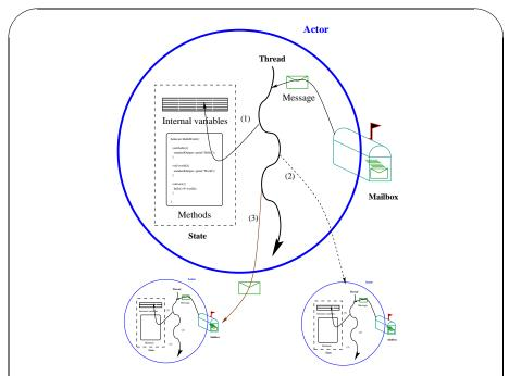
**Fig. 1.1.** In response to a message, an actor can: (1) modify its local state, or (2) create new actors, or (3) send messages to acquaintances.
