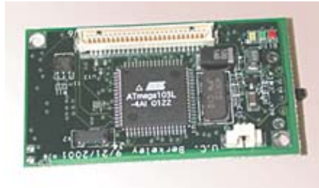
Figure 5: The Mica mote processor board. A sensor board featuring a microphone and a variety of other sensors can be attached, turning the mote into a wireless sensor platform.
