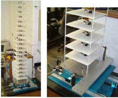
Fig. 2 Sensors are attached to an 18-story building model on a shaking table.
